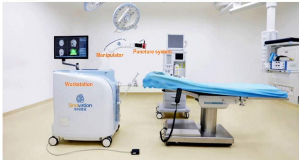
FIGURE 1 The SINO neurosurgical robot, including manipulator, puncture system, workstation and Sinoplan software system
