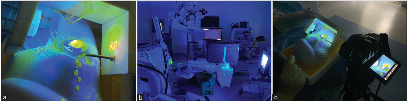
Figure 1: (a) Simulator eye showing extent of fluid droplet spray following emulsification in ultraviolet light, (b) experimental setup for simulator eye with fluorescein stained BSS and ultraviolet light and (c) external digital SLR camera for recording of phacoemulsification and fluid droplet generation
