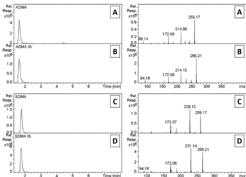
**Fig. 1.** ADMA (Fig. 1A), ADMA internal standard (Fig. 1B), SDMA (Fig. 1C) and SDMA internal standard (Fig. 1D) chromatograms with their mass spectra.
