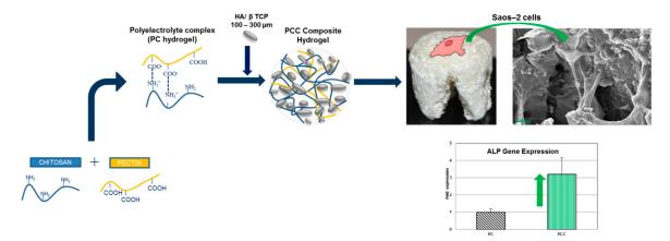
**Figure 5.** Moldable composite scaffold (pectin/chitosan hydrogel + biphasic calcium phosphate particles) for alveolar bone regeneration: the material promotes osteoblast adhesion and proliferation with a 3-fold higher ALP gene expression at one week compared to the control. Reproduced with permission from [225].
