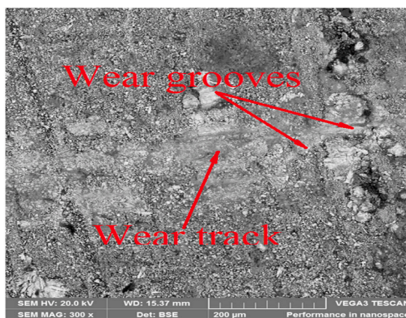
Fig. 22. SEM image of the wear scar on 0.3Zn-7Si 3 N 4 sample.
