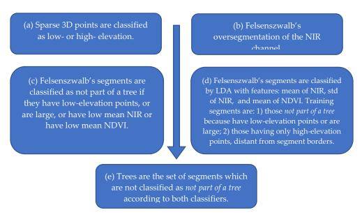
Figure 7. Steps of the tree segmentation algorithm.
