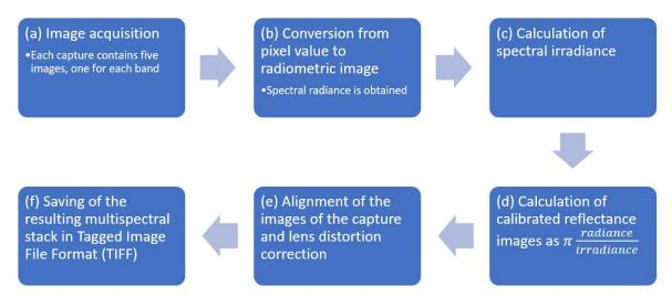
**Figure 6.** Steps of image calibration and alignment.
