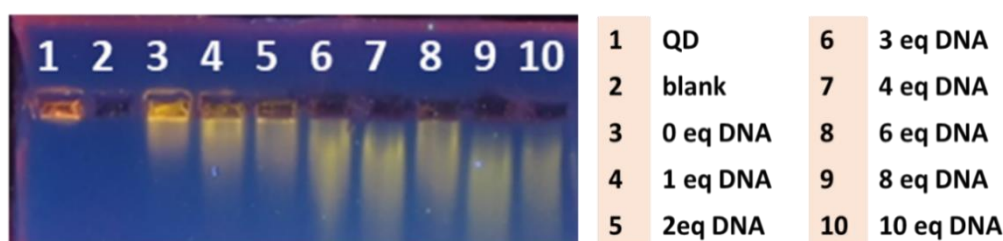
Figure 3. Agarose gel electrophoresis of QDs and QD-DNA conjugates (1% agarose gel, 1 × SB buffer (pH 8.5), 100 V). Stained with thiazole orange aqueous solution. Line 1—freshly prepared QDs alone; 2—DNA alone (blank); 3—QD after the reaction, no DNA was added; 4–10 products of the coupling reaction between QDs and varied concentrations of DNA.
