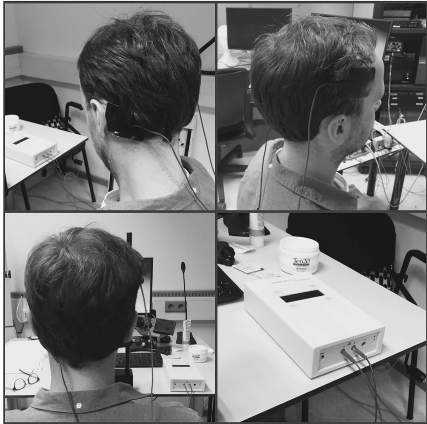
Fig 2. TDCS setup. Anode over F4, cathode over contralateral mastoid.
