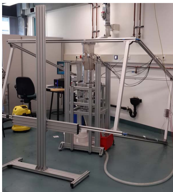
Figure 3. Overview of the 3-D fluidized setup including the sensor array and Helmholtz coil.
