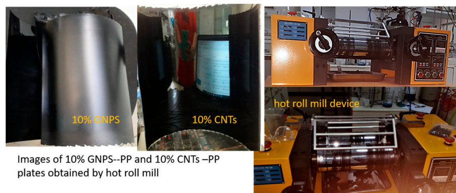
Figure 1. Examples of composite materials panels and photos of the hot roll mill device.
