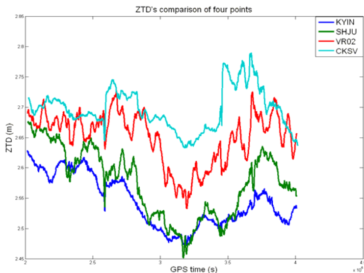
Figure 25. ZTD comparison of e-GPS stations in the north, northwest, southwest, and south during the plum rains.
