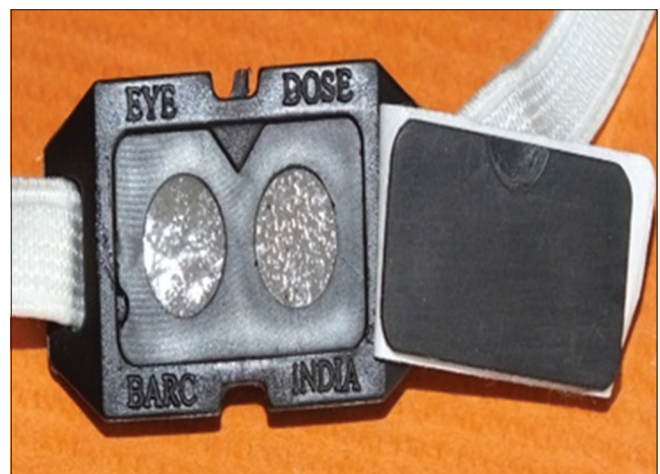
Figure 1: Photograph showing Bhabha Atomic Research Centre-designed eye lens dosimeter used in this study
