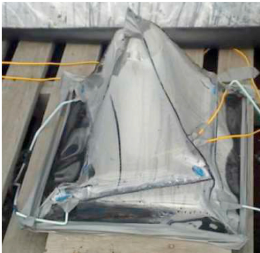
Figure 16. Photographic view of Novel portable pyramid solar still (PSS) which is a portable and flexible solar still and can be inflated wherever required [90].
