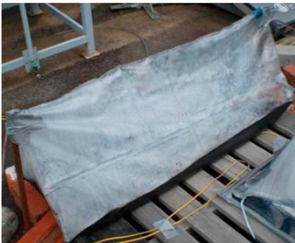
Figure 17. Photographic view of Novel portable Triangular prism solar desalting system with portability benefits which is one of the novel approaches [90].
