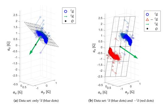
**Figure 2.** Estimated sagittal plane and normal vector extraction from PCA, adding origin symmetric data  $-^{i}\vec{a}$  into the data set of PCA calculation helps to improve the sagittal plane estimation.
