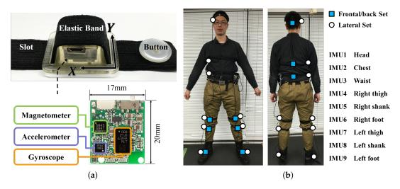
**Figure 4.** Sensor system. (a) WB-4R Inertial Measurement Unit (IMU); (b) Sensor placement. The yellow circles represent the Frontal/back Set, which was attached to the frontal side of lower limbs and the back side of trunk and head. The white circles represent the Lateral Set, which was attached to the lateral side of the body.
