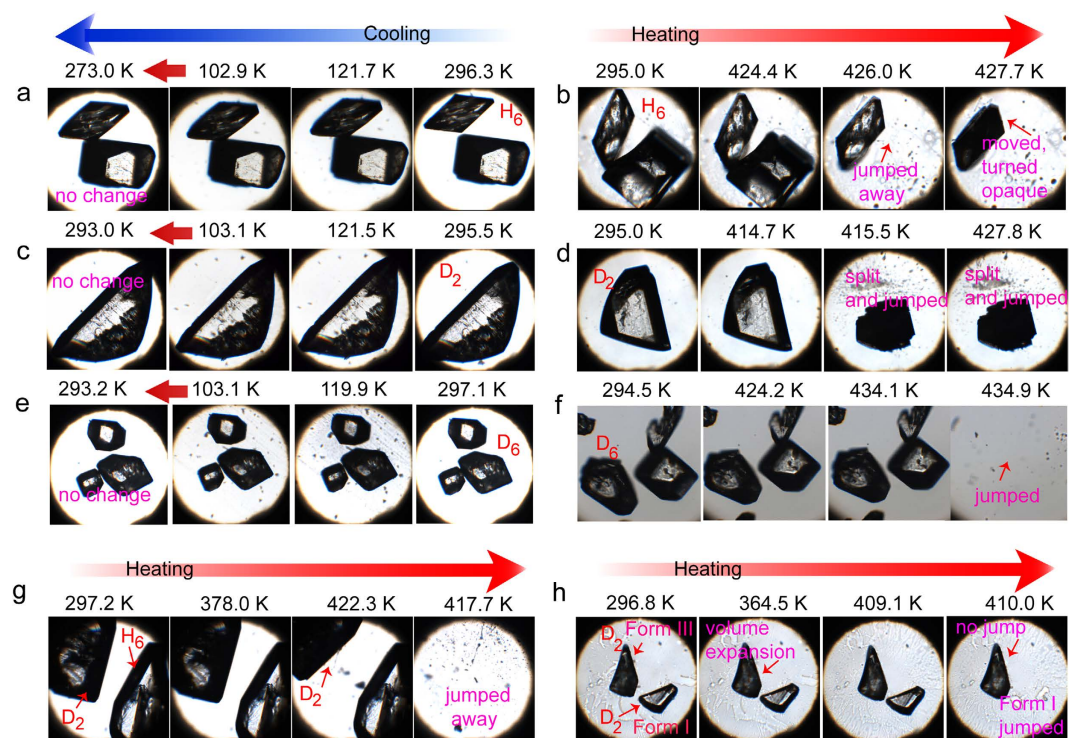
Figure 2. Thermal behavior and thermosalient effect in crystals of protiated and deuterated variants of IMACET recorded by variable-temperature optical microscopy. (a) IMACET-H 6 on cooling by liquid nitrogen. (b) IMACET on heating. (c) IMACET-D 2 on cooling. (d) IMACET-D 2 on heating. (e) IMACET-D 6 on cooling. (f) IMACET-D 6 on heating (the background of this set of images appears darker due to the use of polarizing filter). (g) IMACET and IMACET-D 2 on heating. (h) Form I and form III of IMACET-D 2 on heating.
