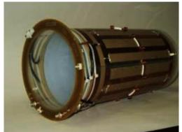
Figure 1: MRI RF coils (adapted from http://198.173.87.9/mri/mri\_litzcagepg.htm)
