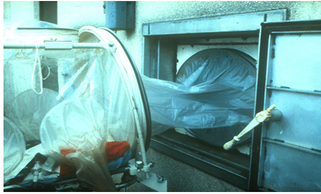
Fig. 4. Docking the stretcher transport isolator at USAMRIID's slammer. Used with permission.
