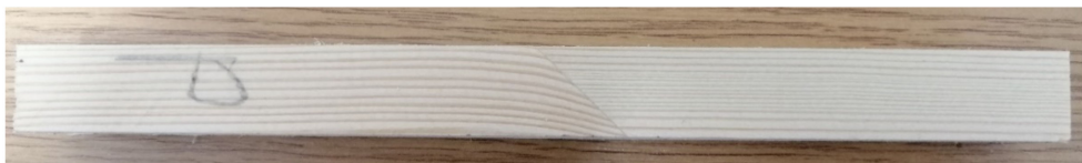
Figure 8. View of the tensile specimen (cross-section approx. 20 × 20 mm).
