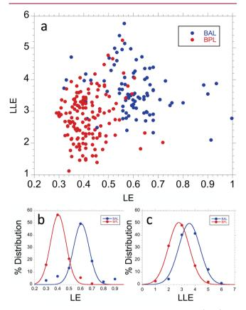
**Figure 3.** Hit distribution against ATX for our boronic acid (BAL) and biophysical libraries (BPL) as a function of ligand efficiency (LE) and lipophilic ligand efficiency (LLE) (a). The BPL has an average LE of 0.41, while the BAL LE averages 0.61 both libraries have a standard deviation of 0.1 (b). The LLE distribution of the libraries are distinct with the BPL library having an average LLE of 2.8 while the BAL library averages 3.6 both libraries have a standard deviation of 1.1 (c).
