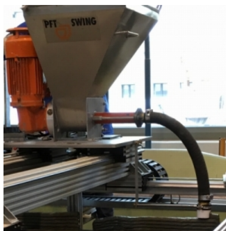
Figure 2. 3D-concrete-printing test device (3DPTD).
