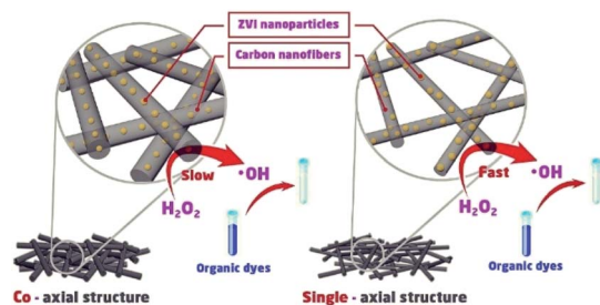
Scheme 1 The speculated degradation mechanism of MB catalysed by as-prepared carbon nanofibrous mats with either the single-axial or co-axial structure.
