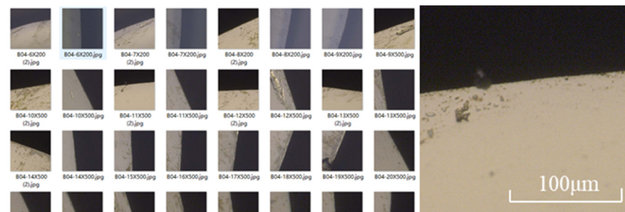
Figure 9. Image of diamond tool defect collected on-machine.
