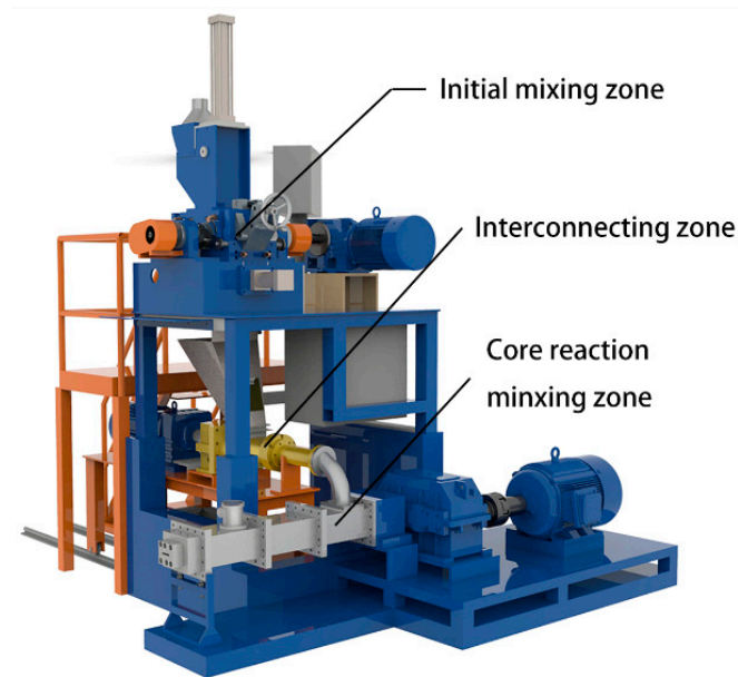
Figure 2. Integral structure of the serial modular continuous mixer.
