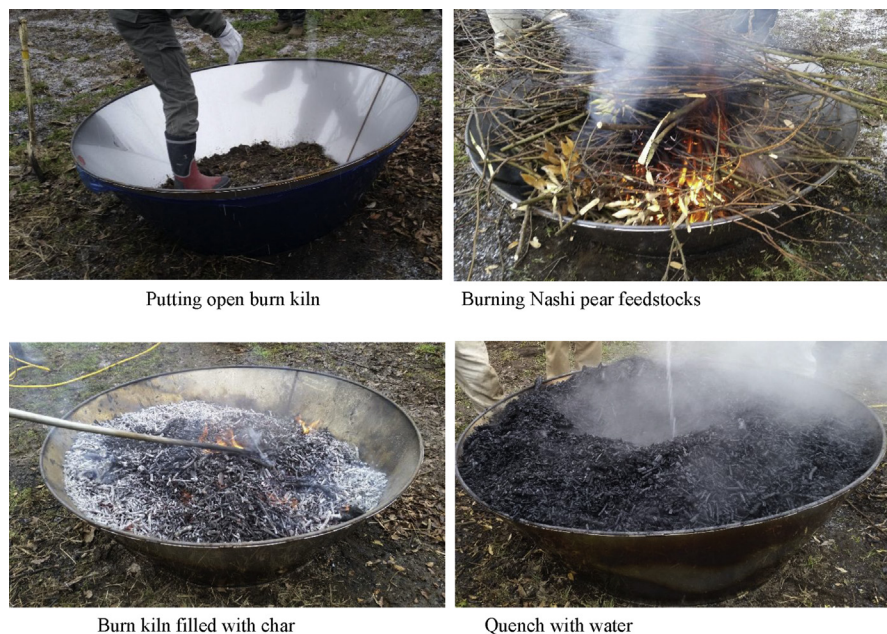
Fig. 1. Making biochar in an open burn kiln using pruning residues of Nashi pear orchard.
