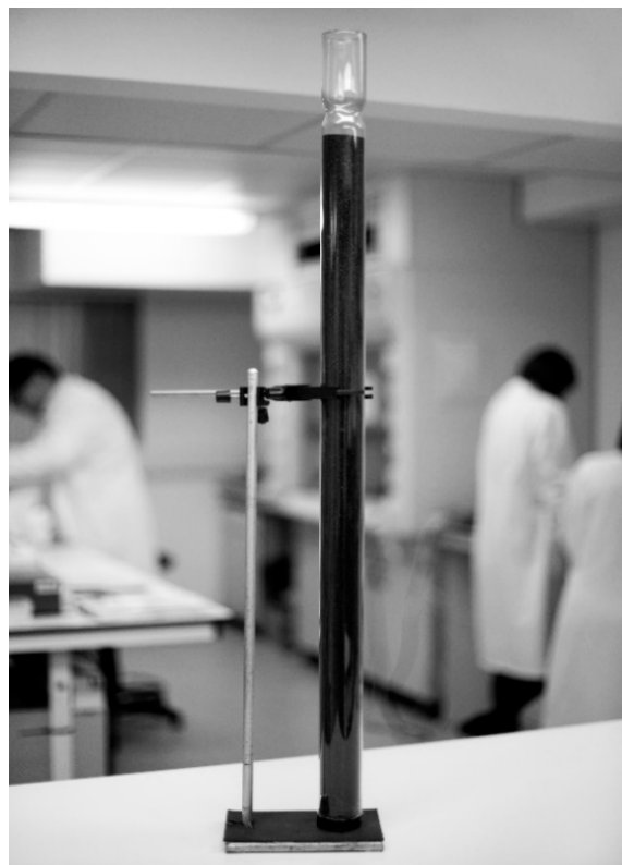
Figure 5. The original glass column filled with charcoal used to prepare phenylalanine-free casein hydrolysate for Sheila's diet.
