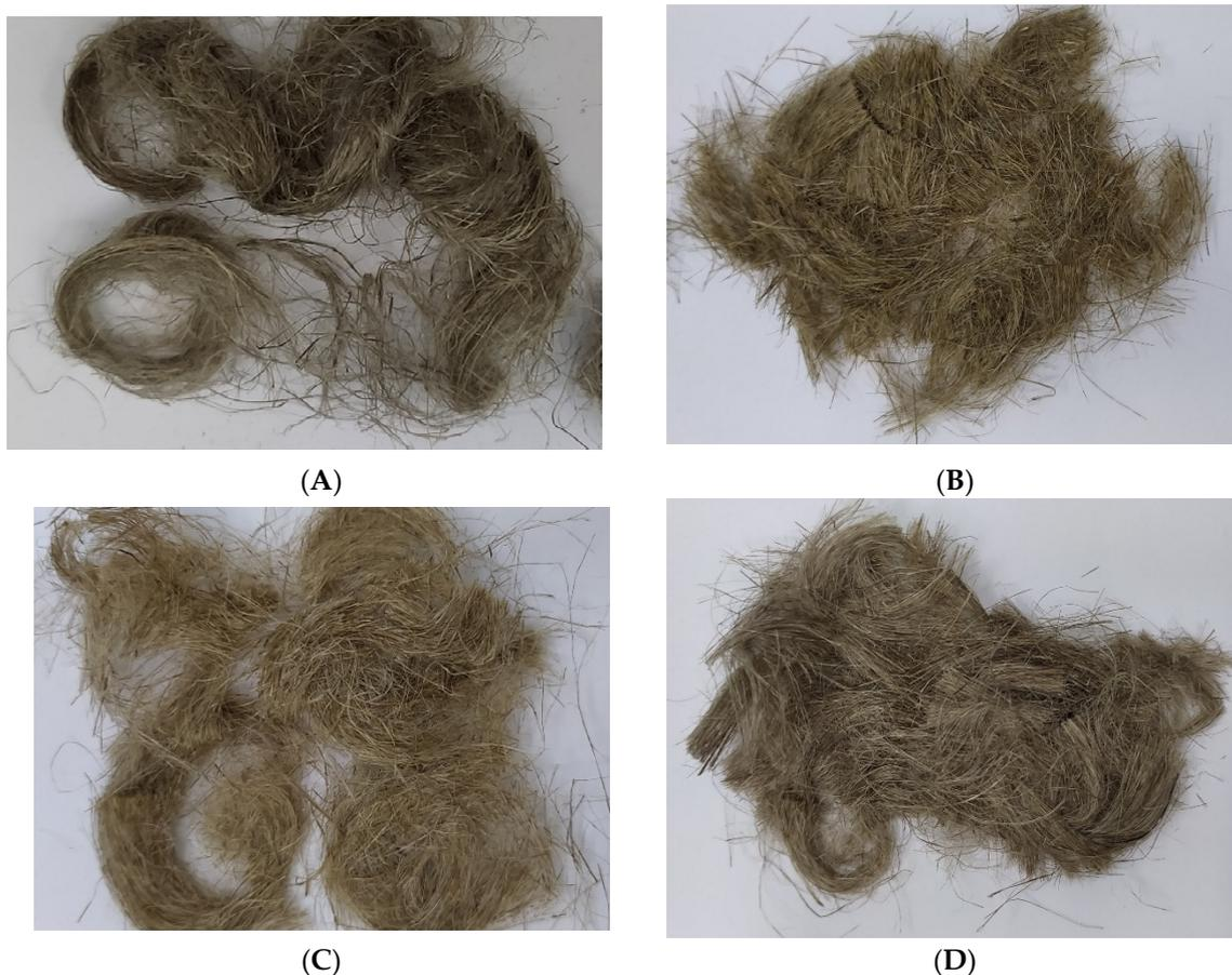
**Figure 17.** Flax fibers tested in the study: (A) NIKE plant fiber, (B) M plant fiber, (C) B plant fiber, and (D) MB plant fiber.
