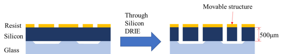
Figure 5. Schematic fabrication process. Through silicon DRIE is applied to the silicon layer of the bonded wafer. The minimum gap of the silicon layer is 25 \mu\text{m} to attain an aspect ratio of 20.
