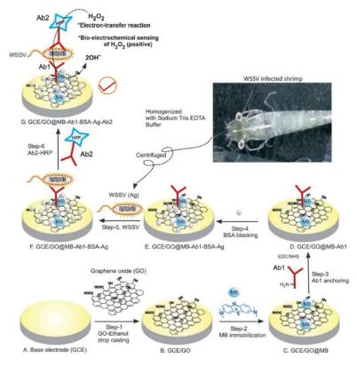
**Figure 5.** Schematic illustration for the development of electrochemical white spot syndrome virus immunosensor using a methylene blue dye (MB) immobilized graphene oxide modified glassy carbon electrode. Reproduced with permission from [76], Copyright Springer Nature, 2017.
