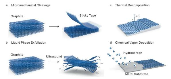
**Figure 1.** Schematic illustration of the graphene and its derivatives synthesis methods. (a) Mechanical exfoliation (b) liquid phase exfoliation, (c) thermal decomposition, and (d) chemical vapor deposition. Reproduced with permission from [23], Copyright Springer Nature, 2017.
