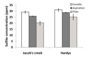
The aspiration analysis was performed as outlined by Iland *et al.* [10] however the suggested concentration of the sodium hydroxide solution was diluted 10 fold in an attempt to achieve greater accuracy in the titration results. Each wine was tested in duplicate.
