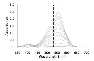
**Figure 8.** Calibration curves obtained at the maximum absorbance and at 532 nm for solutions containing 0–100 ppm of sulfites using a  $7.8 \times 10^{-4}$  mol/L working solution.
