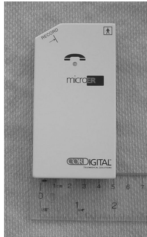
Fig. (2). Transtelephonic Monitors. The device is lightweight and portable. Four recording electrodes are present on the back of the device to permit single lead rhythm strip capture. A record button (top left) is pressed at the onset of symptoms, and the recorded event is transmitted to a base station over an analog phone line.
