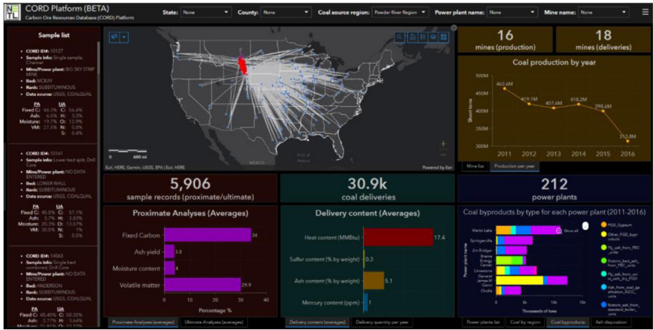
Fig. 2. displays an example and screenshot of the “Infrastructure network” datasets used within a dashboard web application entitled, “CORD Platform”. The map (top center) displays coal delivery pathways extending from mine (black squares) to power plants (blue triangles) and coal samples (red circles) associated with the Powder River (Basin) coal source region. Datasets are summarized within charts, lists, and graphs accordingly.
