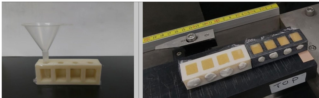
Figure 1. Sample carrier for granular or powdered samples. (A) The compartment openings are covered with XRF film and then the carrier is flipped 90 degrees, filled with resin, sealed, flipped back, and then mounted onto the rails of the Itrax XRF Core Scanner. (B) The whole carrier is scanned in one procedure, but only spectra from the middle of each compartment are used to avoid edge effects and bias from the carrier material.
