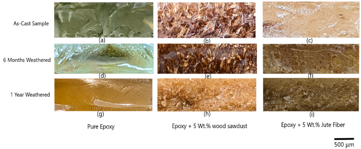
Fig. 7. Fractured surface of Charpy impact test samples.
