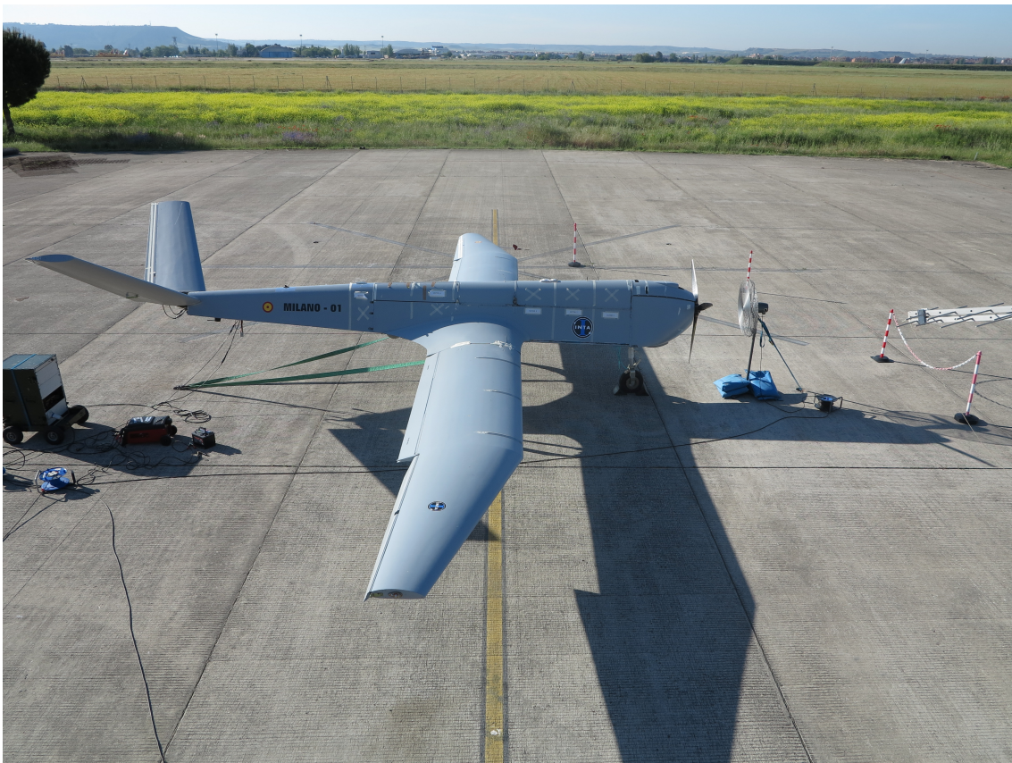
Figure 1. MILANO: a medium altitude long endurance remotely piloted aircraft system development at the National Institute for Aerospace Technology (INTA).
