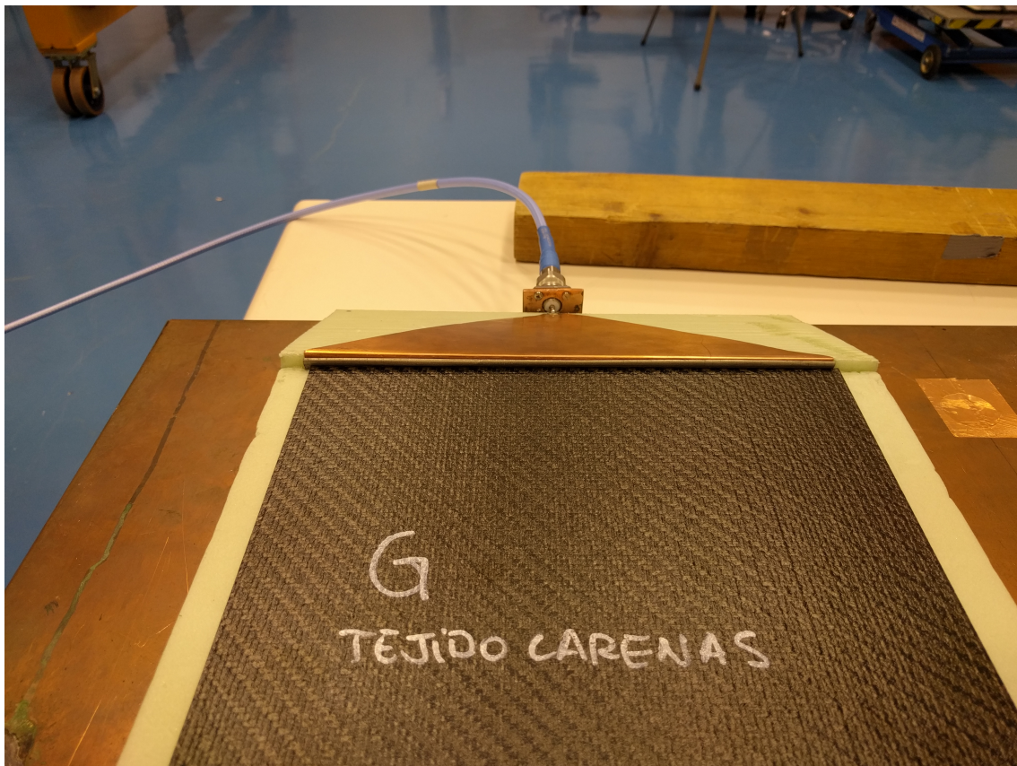
Figure 4. Metallic gasket to achieve a good connection between the triangular transition and the sample.
