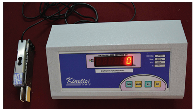
Figure 1: Bite force recorder with biting fork
