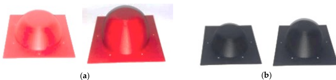
Figure 13. Parts, inferior and superior, of the mould to generate the physical prototypes: (a) Moulds for calibre 1; (b) moulds for calibre 2.
