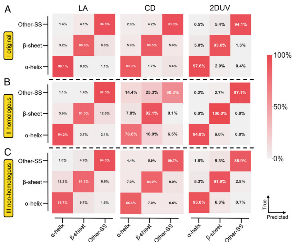
Fig. 4. Confusion matrices of the CNN models after transfer learning to recognize secondary structures of protein segments. The vertical and horizontal axes denote the true and model-predicted categories, respectively. Each matrix element represents the ratio of samples with corresponding categorical labels. Near-unity diagonal values reflect high recognition accuracies. (A) The original set I. (B) The homologous set II. (C) The nonhomologous set III.
