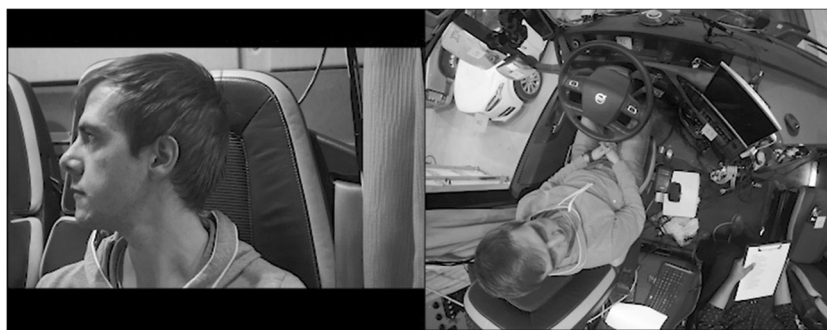
Fig. 2 Video still of the medium-tall driver looking at the right pedestrian mirror (glance location R4) after an instruction from the experimenter. Image published with permission of the participating driver
