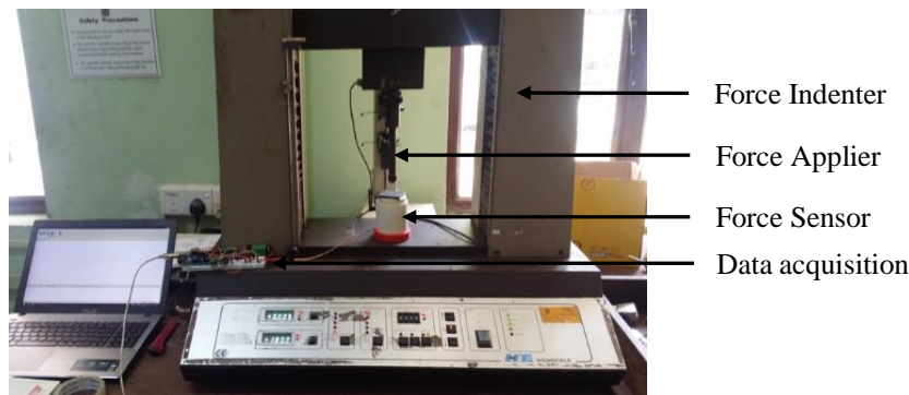
Figure 20. Force indenter is used for sensor characterisation.
