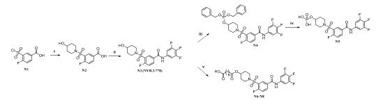
**Scheme 1.** Reagents and conditions. (i) 4-hydroxypiperidine, DIEA, MeCN, 0 °C, 8 h; (ii) 3,4,5-trifluoroaniline, HATU, DIEA, CH<sub>2</sub>Cl<sub>2</sub>, r.t., 8 h; (iii) 1H-imidazole, dibenzyl diisopropylphosphoramidite, 3-chlorobenzoic acid, DCM, 0 °C, 10 h; (iv) H<sub>2</sub>, palladium carbon, THF, r.t., 12 h; (v) various anhydrides, DMAP, Et<sub>3</sub>N, CH<sub>2</sub>Cl<sub>2</sub>, r.t., 10 h.
