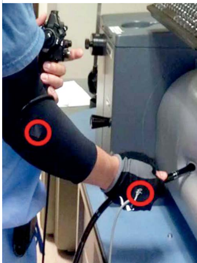
Fig. 2 Subject with magnetic position trackers held in place by custom-made arm sleeve and glove.
