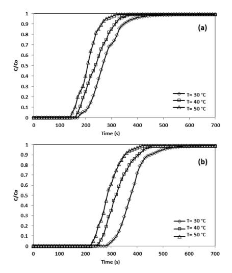
**Figure 13.** Breakthrough curve and effect of temperature (**a**) CNFCM and (**b**) Modified CNFCM in constant P = 1 bar, and 10% CO<sub>2</sub>.
