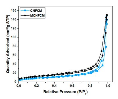
Figure 9. N<sub>2</sub> ads-des isotherm of CNFCM and modified CNFCM.
