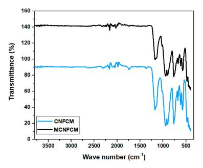
**Figure 10.** FTIR spectrums of CNFCM and modified CNFCM prepared over the following reaction conditions: reaction temperature of 800 °C, furfuryl alcohol flow of 0.08525 mL/min, ferrocene catalyst concentration of 2.21 g.
