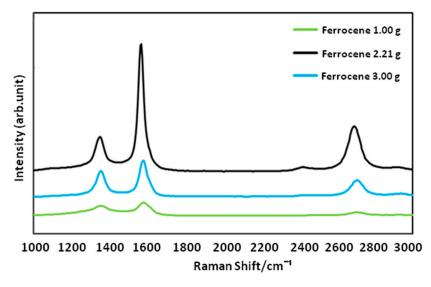
Figure 7. Raman spectra of CNFs prepared with different ferrocene concentrations.
