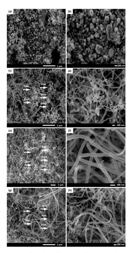
Figure 4. FE-SEM images of the carbon nanofiber-coated monoliths (CNFCMs) synthesized at various temperatures (a and b) 600 °C, (c and d) 700 °C, (e and f) 800 °C, (g and h) 900 °C. Red arrow: iron catalyst.
