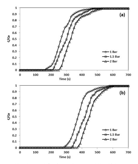
**Figure 14.** Breakthrough curve and effect of pressure (**a**) CNFCM and (**b**) modified CNFCM in constant  $T = 30 \degree C$ , Flow = 50 mL/min, and 10% CO<sub>2</sub>.
