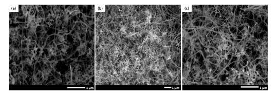
**Figure 6.** FE-SEM images of CNFs prepared with different ferrocene concentrations: (**a**) ferrocene (1.00 g), (**b**) ferrocene (2.21 g), (**c**) ferrocene (3.00 g).
