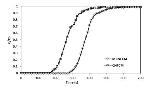
**Figure 15.** Breakthrough curves adsorption of CNFCM and modified CNFCM in constant 40% CO<sub>2</sub>, T = 30 °C, P = 1 Bar.
