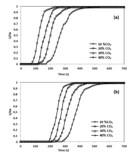
**Figure 12.** Breakthrough curve and effect of initial concentration (**a**) CNFCM and (**b**) modified CNFCM in constant  $T = 30 \degree C$ , P = 1 bar and Flow = 50 mL/min.
