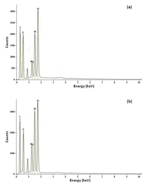
Figure 8. EDX analysis of (a) CNFCM and (b) modified CNFCM.
