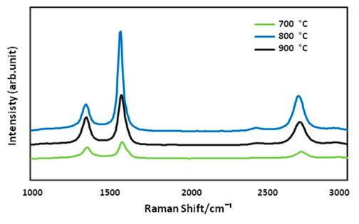
Figure 5. Raman spectra of the CNFCMs synthesized at various temperatures.
