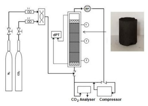
Figure 1. A graphical illustration of the experimental set-up for adsorption of carbon dioxide (CO<sub>2</sub>).
