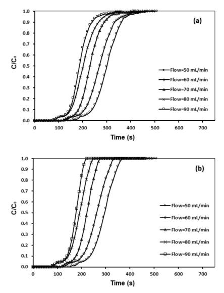
**Figure 11.** Breakthrough curve and effect of flow rate of (**a**) CNFCM and (**b**) modified CNFCM in constant T = 30 °C, P = 1 bar and 10% CO<sub>2</sub>.
