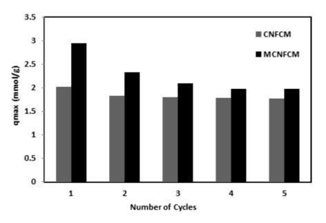
Figure 16. Cyclic adsorption of CO<sub>2</sub> of CNFCM and MCNCM (40% CO<sub>2</sub>, T = 30 °C, P = 1 Bar).
