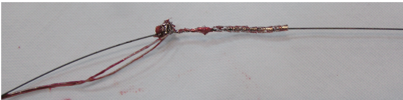
Figure 4. The externalized stent showed severe shape deformation and structural distortion.
