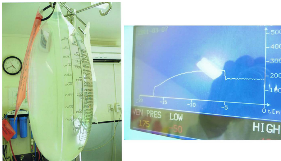
Figure 4 A saline bag after a simulation of circumstances surrounding the deceased's last dialysis treatment. The weight of the bag was 4kg, and venous pressures with a pump speed of 200mL/min rose to only just higher than 200mmHg during this exercise.
