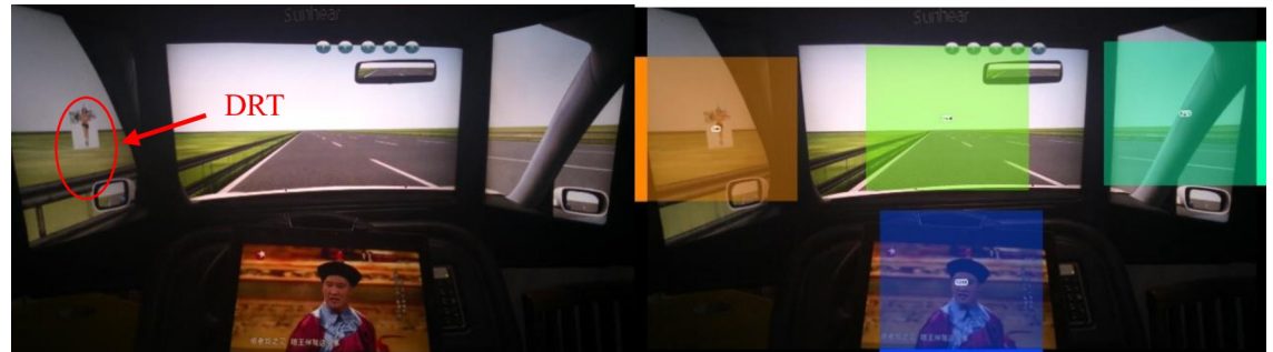
Fig 2. Division of area of interest of the portable eye tracker and collection of fixation duration indicators.
