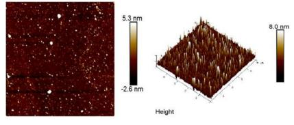
Figure 2. AFM analysis of IOPS. Reproduced with permission [83].
