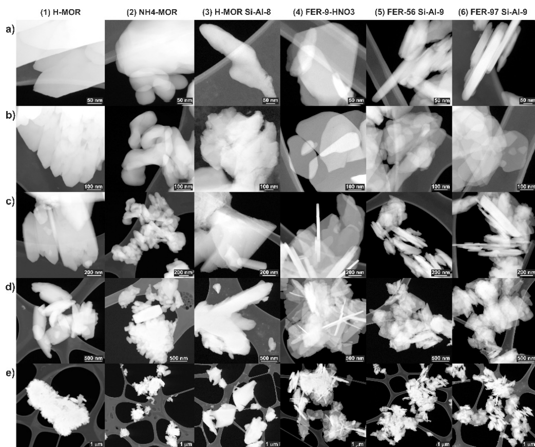
Figure 13. STEM overview and detail aspect images (a–e) of the zeolite morphology: mordenite (MOR, samples 1–3, columns 1–3, resp.), ferrierite (FER, samples 4–6, columns 4–6) samples of various Si/Al ratio.
