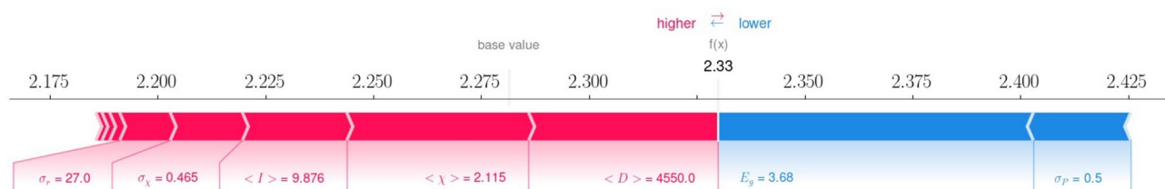
Fig. 6. SHAP force plot showing features impact on model prediction corresponding to ZnS which has the median RI value among unseen data (experimental RI: 2.35, prediction RI: 2.33).
