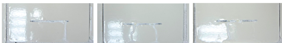
Figure 3. The appearance of the polyester coating near the scribe after the NSS test at 750 h.
