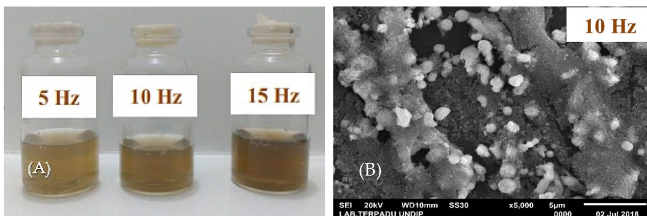
Figure 10. (A) Zn nanoparticles prepared using pulsed laser ablation of Zn in deionised water at different pulse frequencies of 5 Hz (light brown), 10 Hz (medium brown), and 15 Hz (dark brown). (B) Scanning electron microscopy images showing the morphology of dried Zn nanoparticles at a pulse repetition rate of 10 Hz. Adapted with permission from Ref. [124]. Copyright 2019, IOPscience.
